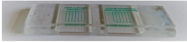
Figure 1: Mc Master Counting chamber. Quantification of the worm eggs infection (Source: Fair Poultry)
